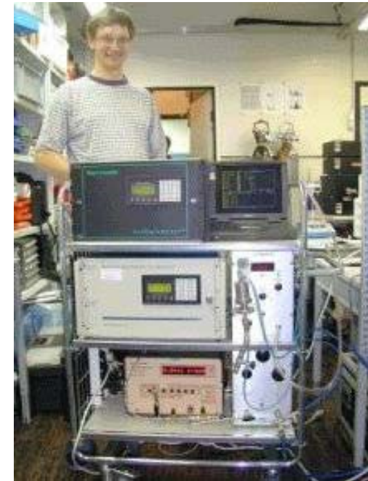
Facility for measuring the size distribution of black carbon in real time
